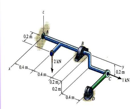
Given: A rod is supported by a ball-and-socket joint at A, a journal bearing at B and a short link at C. Assume the rod is properly aligned.
