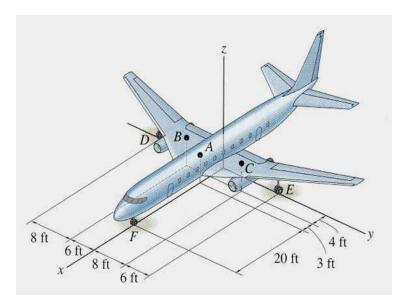
The weights of the fuselage and fuel act through A, B, and C. How will we determine the reactions at the wheels D, E and F?
