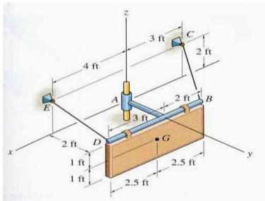
A 50 lb sign is kept in equilibrium using two cables and a smooth collar. How can we determine the reactions at these supports?
