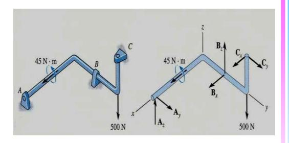
A single bearing or hinge can prevent rotation by providing a resistive couple moment. However, it is usually preferred to use two or more properly aligned bearings or hinges. Thus, in these cases, only force reactions are generated and there are no moment reactions created. Explanation
