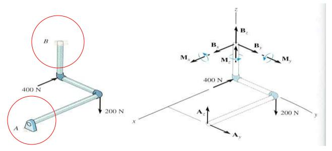
Redundant Constraints: When a body has more supports than necessary to hold it in equilibrium, it becomes statically indeterminate.
