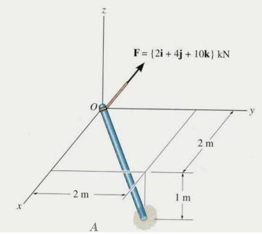
EXAMPLE (continued)  $r_{0A} = \{2i + 2j - 1k\} \text{ m}$  $r_{0A} = (2^2 + 2^2 + 1^2)^{1/2} = 3 \text{ m}$  $F = \{2i + 4j + 10k\}$ kN  $F = (2^2 + 4^2 + 10^2)^{1/2} = 10.95 \text{ kN}$  $F \cdot r_{OA} = (2)(2) + (4)(2) + (10)(-1) = 2 \text{ kN} \cdot \text{m}$  $\theta = \cos^{-1}\{(\mathbf{F} \bullet \mathbf{r}_{OA})/(F r_{OA})\}$
