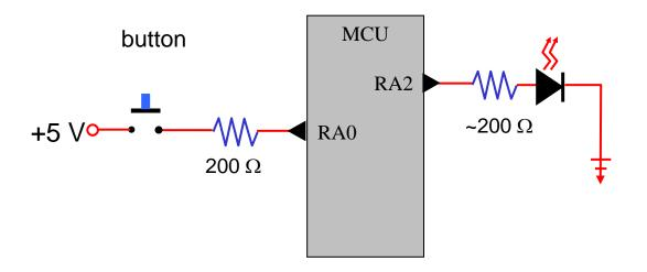
A. When the button is up, RA0 is floating. Random noise can set it high. Added a resistor keeps RA0 grounded when button is up. When button is pressed, do have a current through R. Need R big to keep current low.
